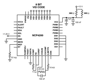
Figure 4. Closed-Loop Output Voltage Accuracy
