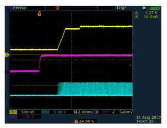
Figure 9. Overcurrent Latchoff Waveforms
