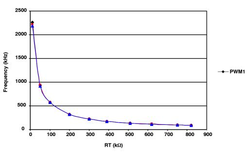
Figure 3. Master Clock Frequency vs. RT
