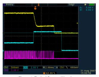
Figure 8. Typical Startup Waveforms
