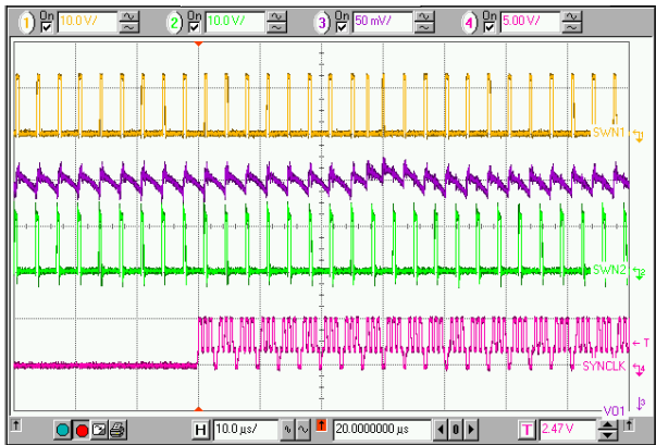
Top to Bottom: SWN_Slave, Vo_Slave, SWN_Master, Sync_clk
