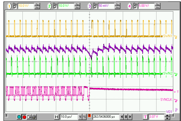
Top to Bottom: SWN_Slave, Vo_Slave, SWN_Master, Sync_clk
