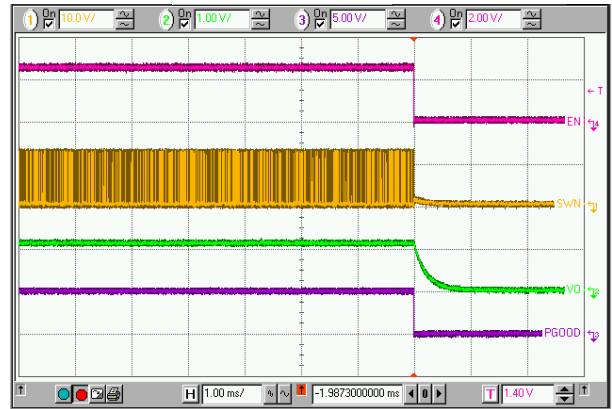
Top to Bottom: EN, SWN, Vo, PGOOD Figure 11. Powerdown Sequence
