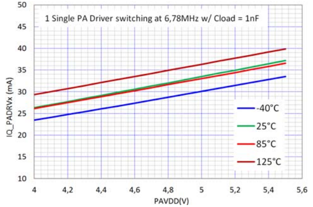
Figure 35. Current Consumption vs. PAVDD per PA Driver w/ C_{load} = 1\text{ nF} and Fast Mode
