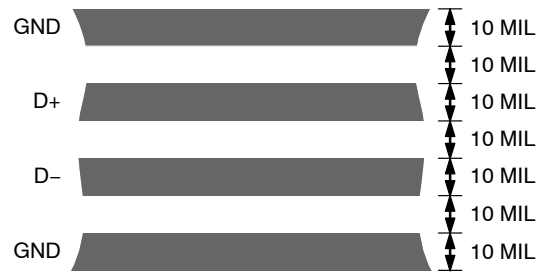
Figure 17. Arrangement of Signal Tracks
