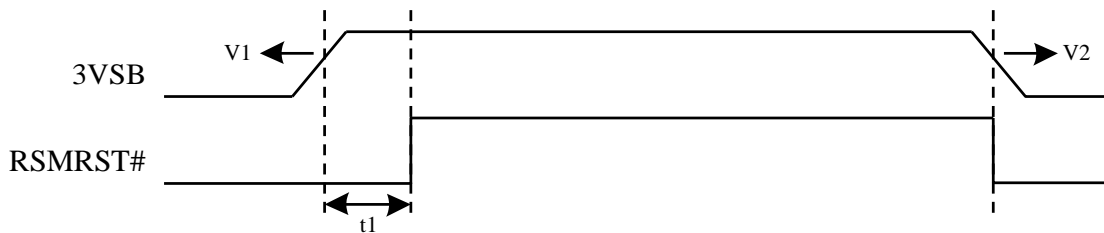
Figure 14-5 Mechanism of Resume Reset Logic
