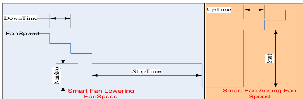
Figure 6-1 SMART FAN™ IV Control Parameters
