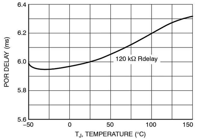
Figure 8. POR Delay vs. Temperature, 120 kΩ Rdelay
