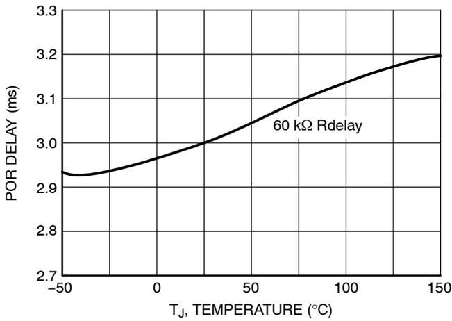
Figure 7. POR Delay vs. Temperature, 60 kΩ Rdelay
