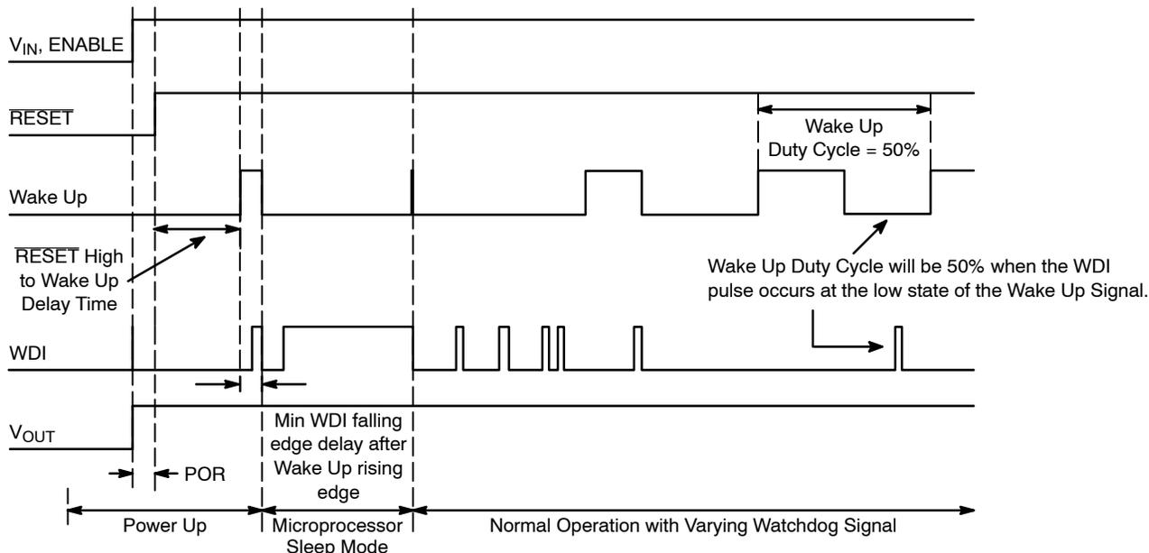
Figure 2. Power Up, Sleep Mode and Normal Operation
