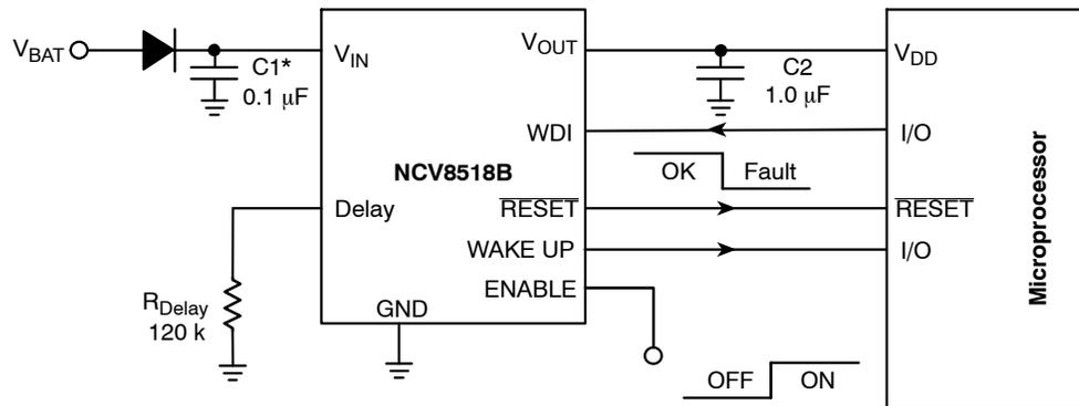
\*C1 required if regulator is located far from power supply filter. If extremely fast input voltage transients are expected then appropriate input filter must be used. The filter can be composed of several capacitors in parallel.
