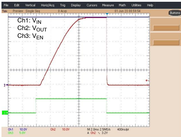
Figure 12. Turning on a Single Output with EN Pin
