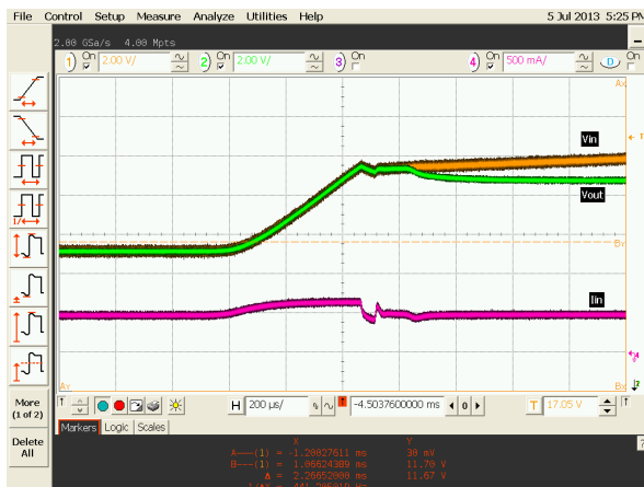
Figure 10 Input Transient Response
