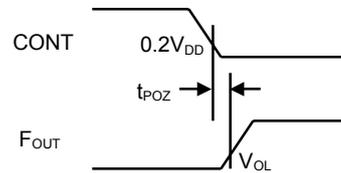
(3) Output Enable Time ( $C_L=15\text{pF}$ )
