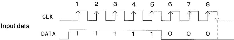
(The system control data is written into the internal register with the falling edge of the 8th clock.)
