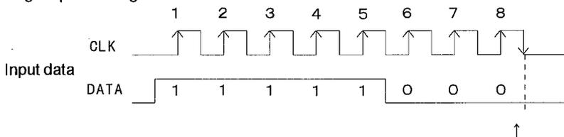
(The timer data is written into the internal register with the falling edge of the 8th clock, and the divider starts operation.)
