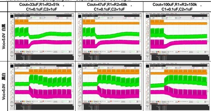
DC level will change by APL fluctuation at the black-and-white change. The rate of change of the DC level is dependent on the capacitance value of Cout.
