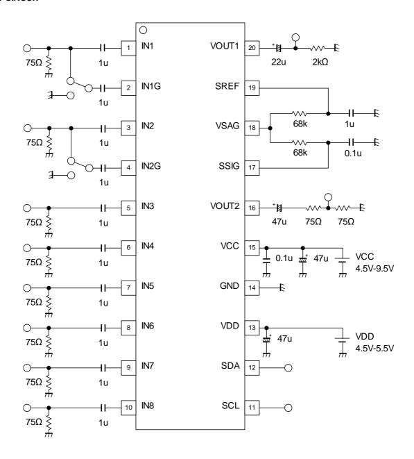
Note) NJW1341 has possibilities that decrease in the capacitance in low-frequency band when the ceramic capacitor is used (pin16). It is a possibility that the sag is generated when the ceramic capacitor decreases capacity. Please verify it in consideration of the capacity drop of the ceramic capacitor.
