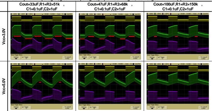
If the power supply voltage is low, if the output capacitor is small, to prevent signal clipping beyond the dynamic range of the OUT terminal, sag correction function stops.
