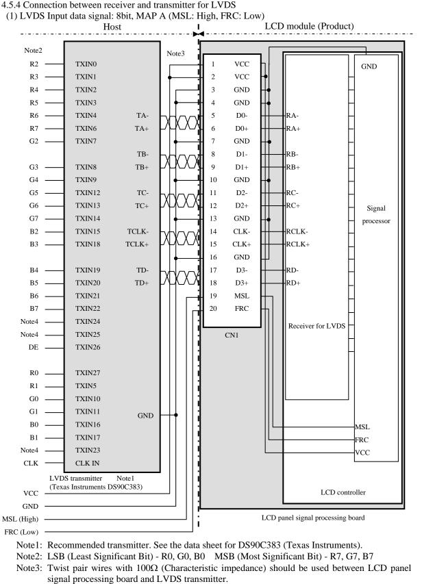
Note4: Input signals to TXIN23, TXIN24 and TXIN25 are not used inside the product, but do not keep TXIN23, TXIN24 and TXIN25 open to avoid noise problem.
