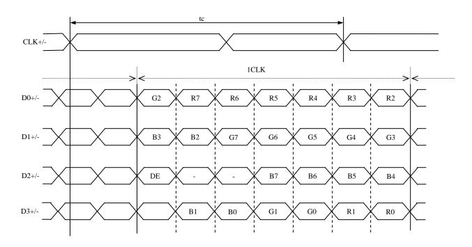
(2) LVDS Input data signal: 8bit, MAP B (MSL: Low or Open, FRC: Low)
