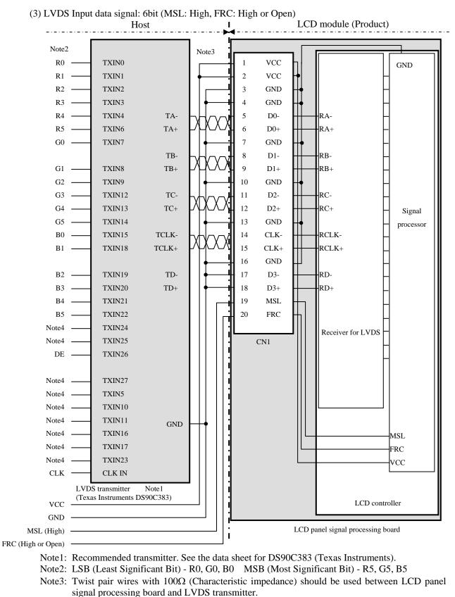
Note4: Input signals to TXIN24, TXIN25, TXIN27, TXIN5, TXIN10, TXIN11, TXIN16, TXIN17 and TXIN23 are not used inside the product, but do not keep TXIN24, TXIN25, TXIN27, TXIN5, TXIN10, TXIN11, TXIN16, TXIN17 and TXIN23 open to avoid noise problem. 5 5
