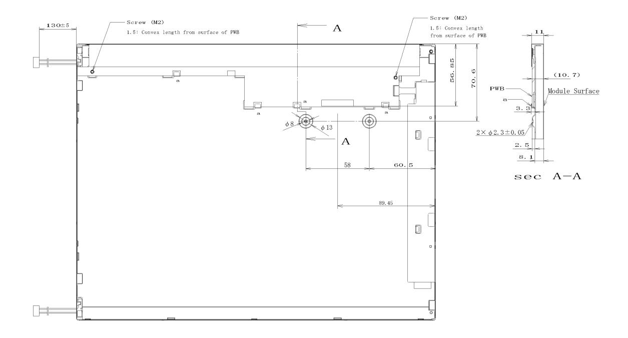
Note1: Not shown tolerances of the dimensions are ±0.5mm. Note2: The values in parentheses are for reference. Note3: The torque for mounting screw should never exceed 0.34N·m.
