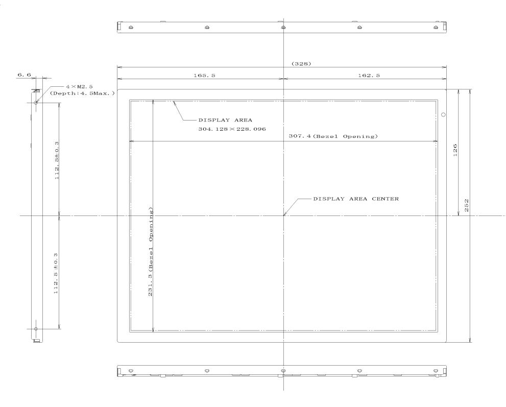
Note1: Not shown tolerances of the dimensions are  $\pm 0.5$ mm. Note2: The values in parentheses are for reference. Note3: The torque for mounting screw should never exceed 0.34N·m.
