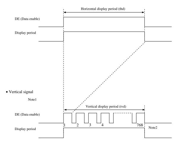
Note1: This diagram indicates virtual signal for set up to timing. Note2: See "**4.8.3 Input signal timing chart**" for numeration of pulse.
