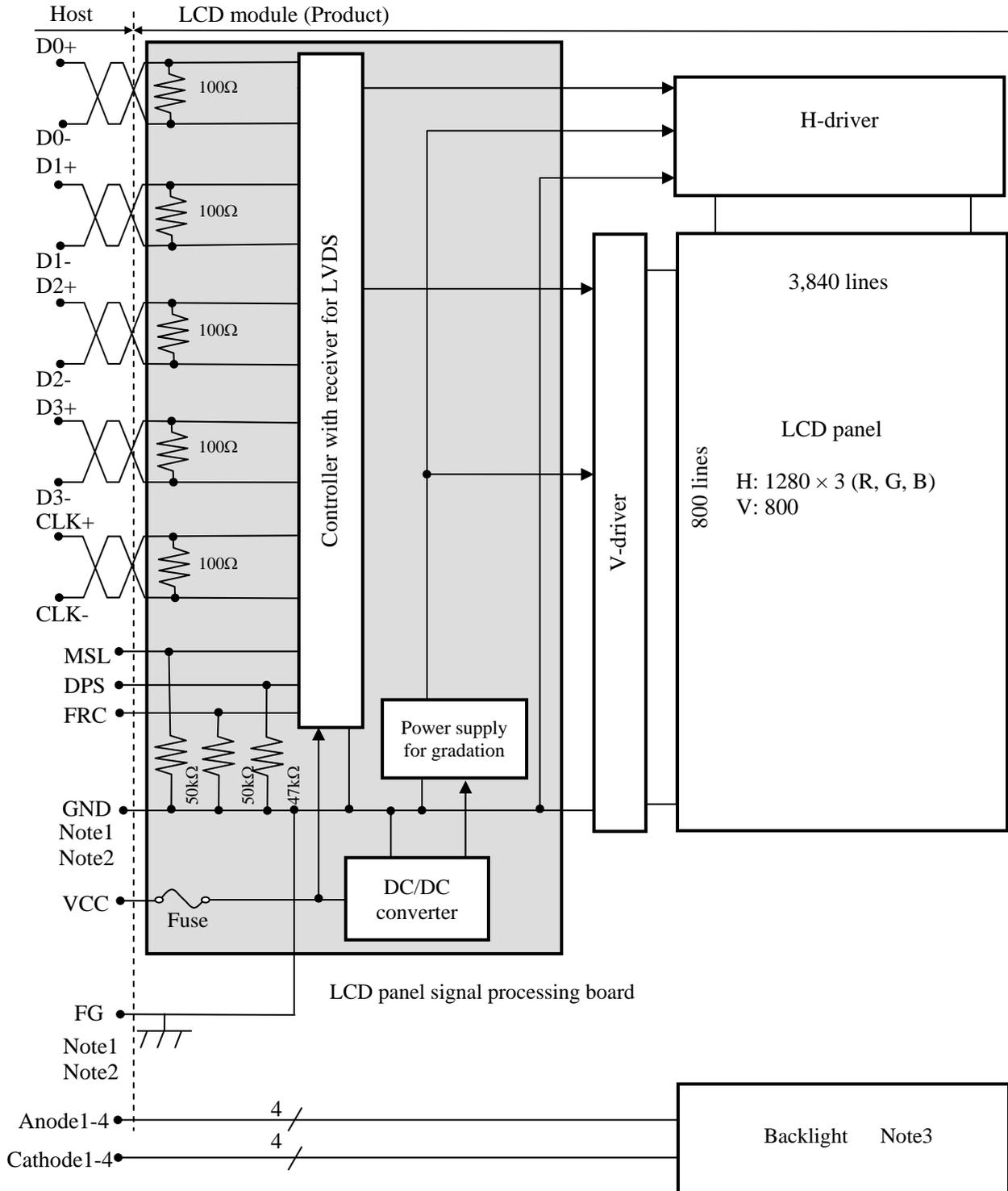
Note1: Relations between GND (Signal ground) and FG (Frame ground) in the LCD module are as follows.
