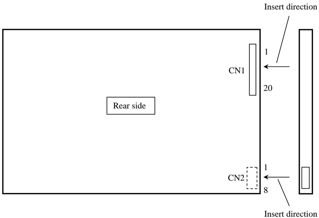
4.5.4 Connection between receiver and transmitter for LVDS
