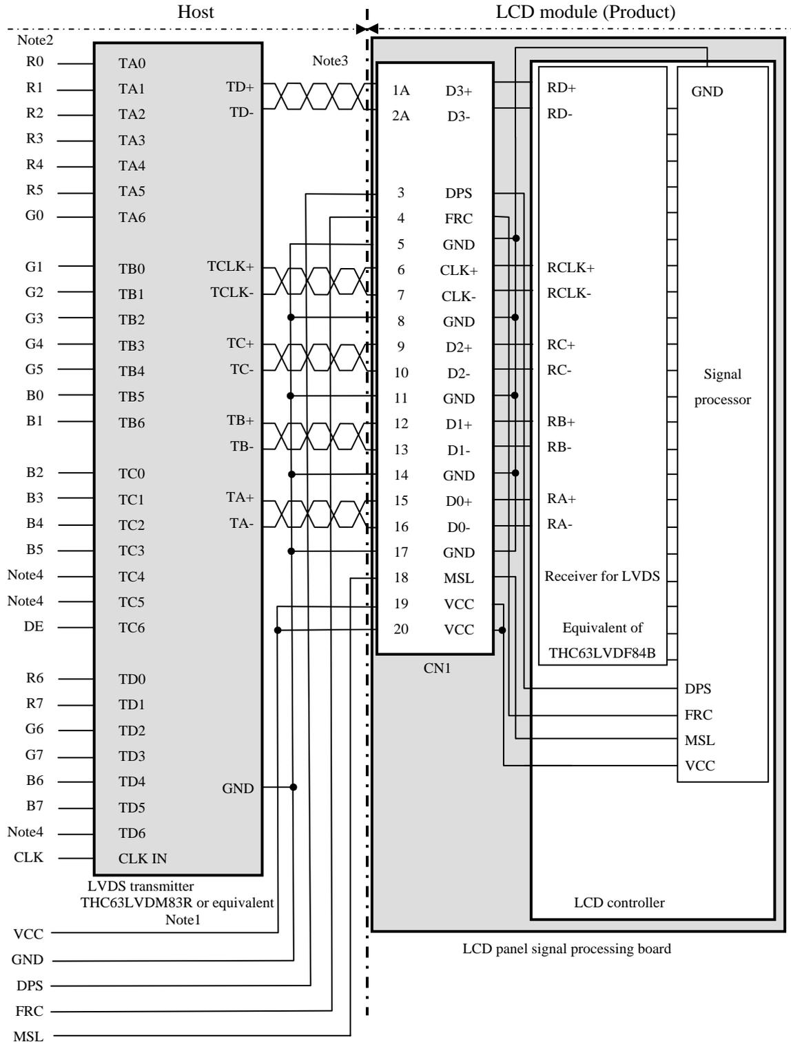
Note1: Recommended transmitter: THC63LVDM83R (THine Electronics Inc.) or equivalent
