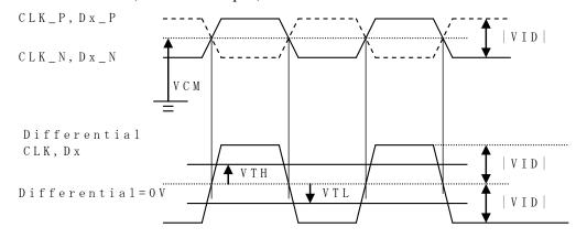
$\begin{array}{l} CLK\_P,\ CLK\_N \\ Dx\_P,\ Dx\_N \quad \ \ x = 0,1,2,3 \\ |VID| = |^{**}\_P^{-**}\_N| \\ VCM = (^{**}\_P^{+**}\_N)/2 \end{array}$
