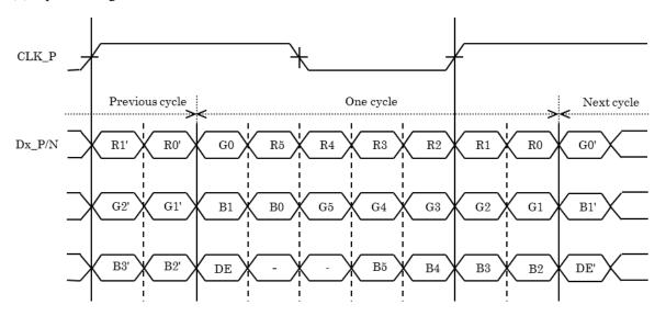
Note1: LSB (Least Significant Bit) – R0, G0, B0 MSB (Most Significant Bit) – R5, G5, B5
