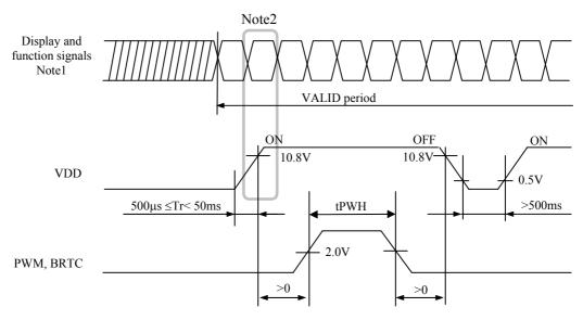
Note1: These are the display and function signals for LCD panel.
