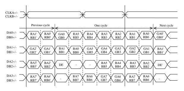
Note1: LSB (Least Significant Bit) – R0, G0, B0 MSB (Most Significant Bit) – R7, G7, B7
