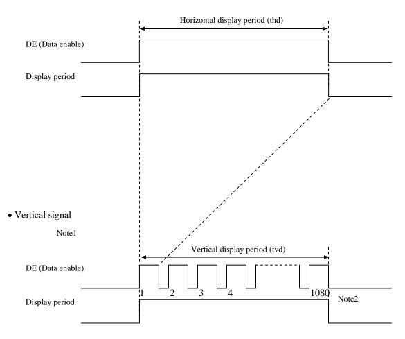
Note1: This diagram indicates virtual signal for set up to timing. Note2: See "**4.8.3 Input signal timing chart**" for the pulse number.
