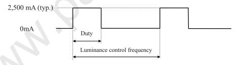
Duty: At the maximum luminance control 100% to at the minimum luminance control 1%. Luminance control frequency: 270Hz (typ.)
