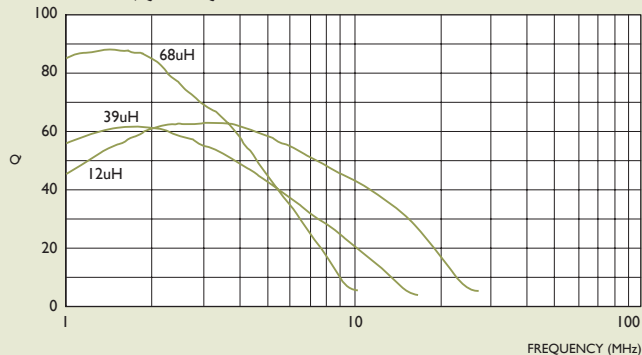
NL453232, Q vs. FREQUENCY CHARACTERISTICS
