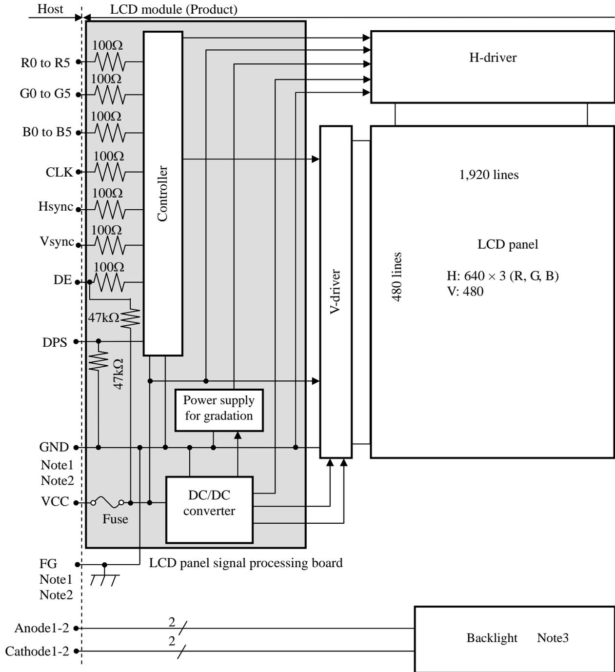
Note1: Relations between GND (Signal ground) and FG (Frame ground) in the LCD module are as follows.
