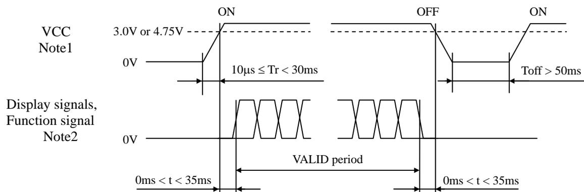
Note1: In terms of voltage variation (voltage drop) while VCC rising edge is below 3.0V in "VCC = 3.3V" or 4.75V in "VCC = 5.0V", a protection circuit may work, and then this product may not work.
