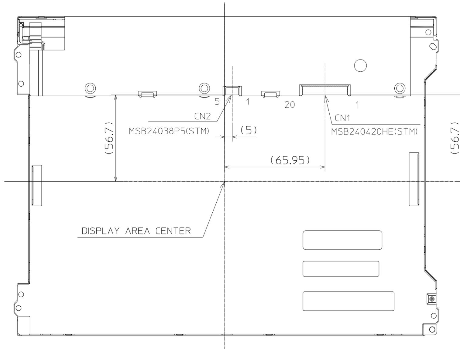
Note1: The torque for product mounting screws must never exceed 0.392N·m. And the length of product mounting screws must be  $\leq 4.5$  mm.
