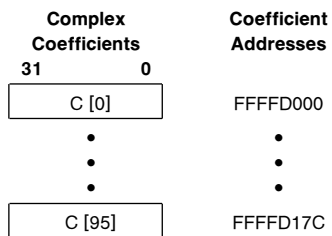
FIGURE 2-8. On-Chip RAM Array Address Map
