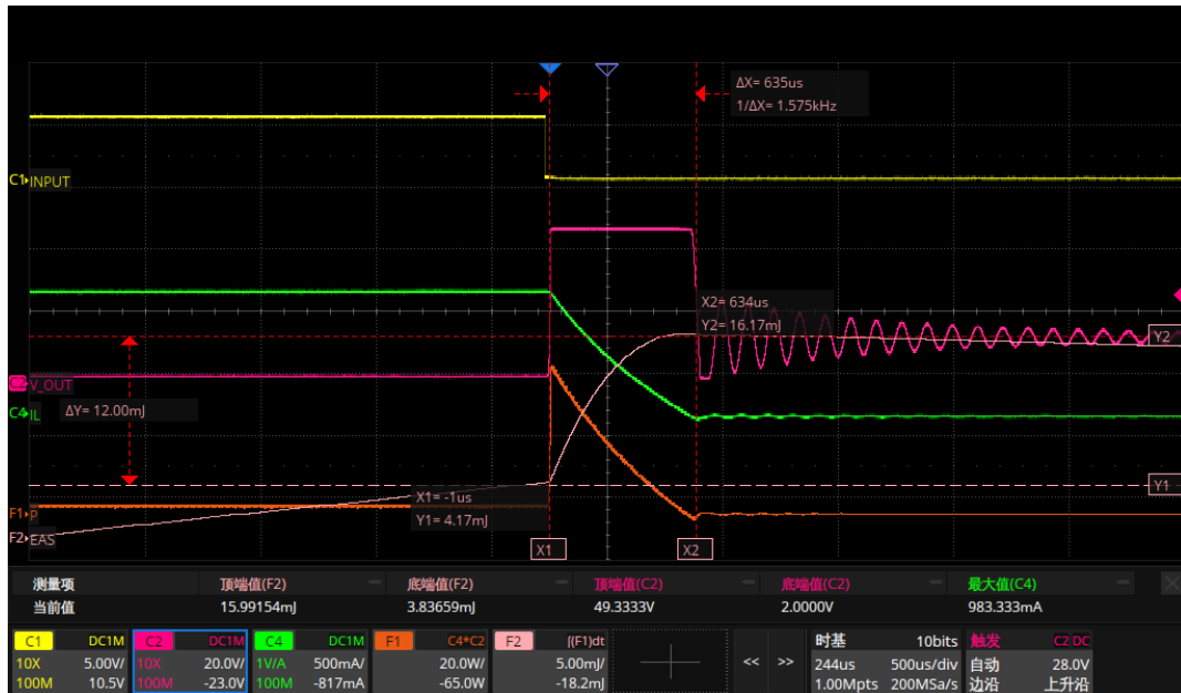
Figure 8.3 LSD Clamped energy actual test waveform
