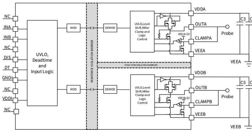
Figure 6.16 Channel to Channel Delay Match Test Circuit
