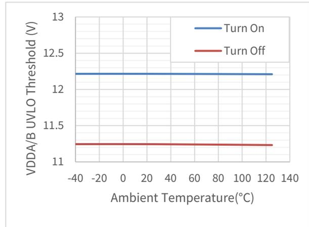
Figure 6.6 6602MC VDDA/B UVLO Threshold vs Temperature
