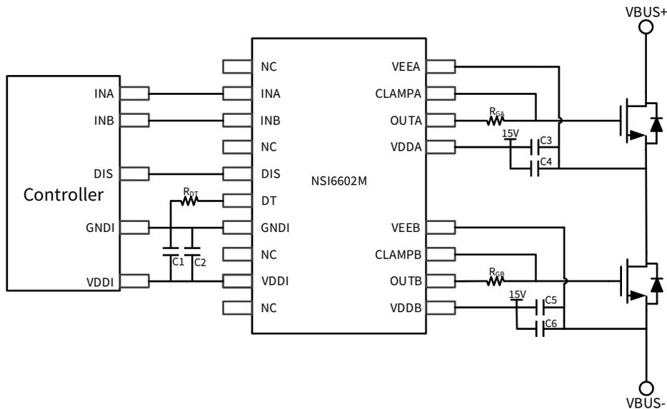
Figure 9.1 Typical Half-Bridge Application Schematic
