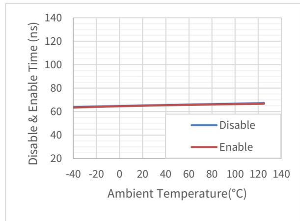
Figure 6.12 Disable & Enable Time vs Temperature
