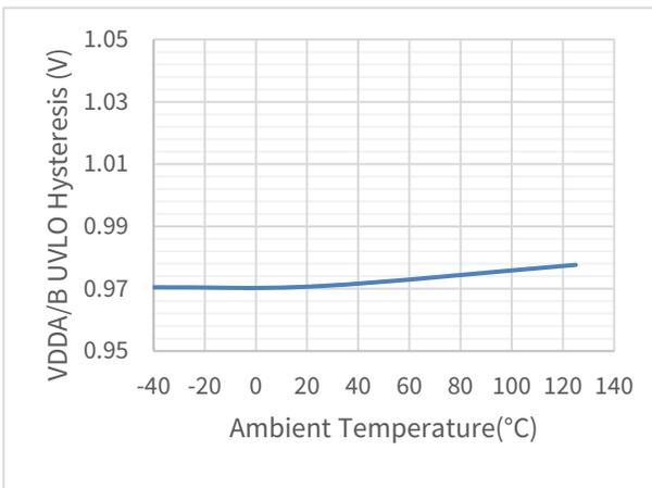
Figure 6.7 6602MC VDDA/B UVLO Hysteresis vs Temperature
