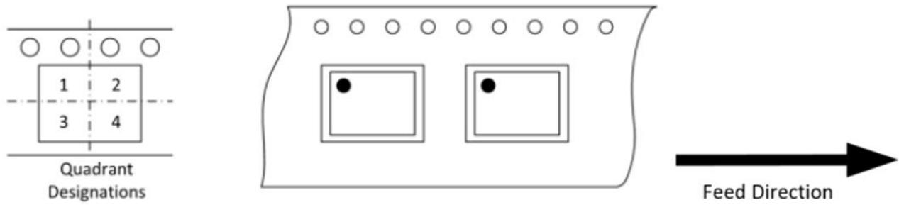
Figure 13.3 Quadrant Designation for Pin1 Orientation in Tape
