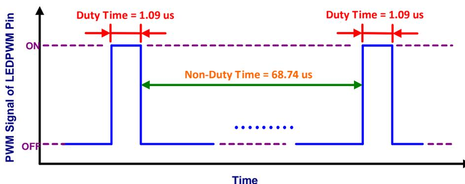
The same, when PWM frequency is 14.32 KHz, and PWM duty of LEDPWM is 256 (Reading the register “RDDISBV[7 : 0]” = FFh), then the duty time can be estimated as shown in below :
