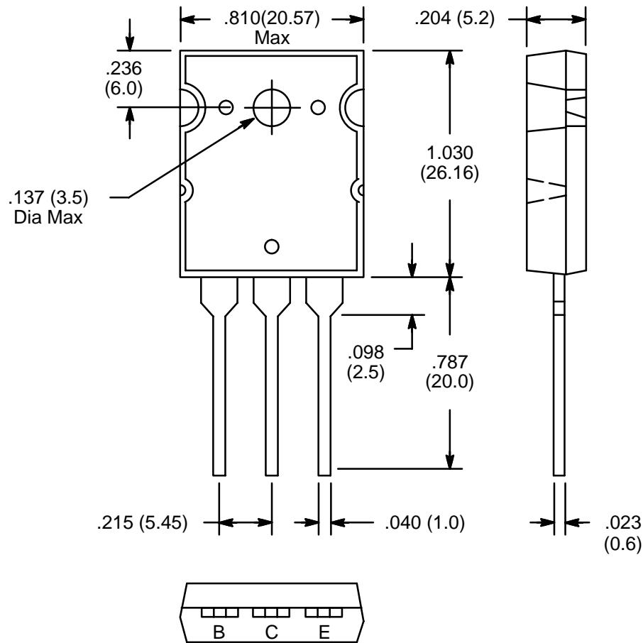
**Note:** Collector connected to heat sink.
