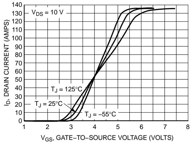
Figure 2. Transfer Characteristics
