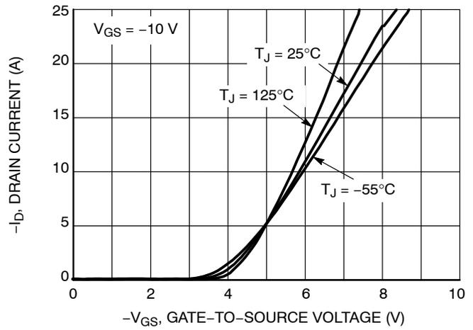
Figure 2. Transfer Characteristics
