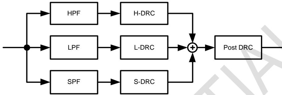
**Figure 17. Block Diagram of Dynamic Range Control**
