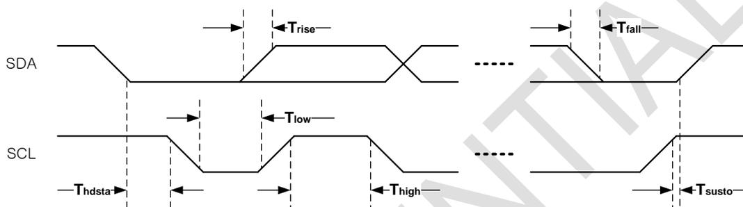
Figure 3. I<sup>2</sup>C Mode Timing
