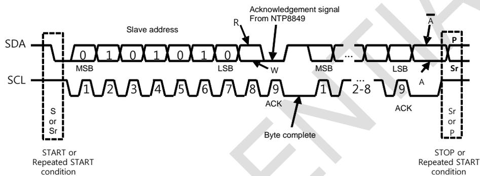
Figure 5. Basic Signaling Elements of I<sup>2</sup>C Bus
