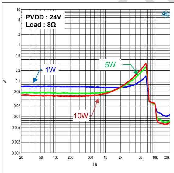
Total Harmonic Distortion + Noise vs. Frequency, BTL D-BTL Mode Configuration, 6Ω
