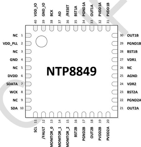
( 40 pin SAW QFN 6mm x 6mm Package )
