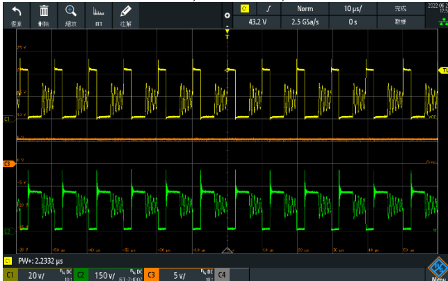
CH1: VDS 20V/div, CH2: Pri_VDS 150V/div, CH3: VDD 5V/div
