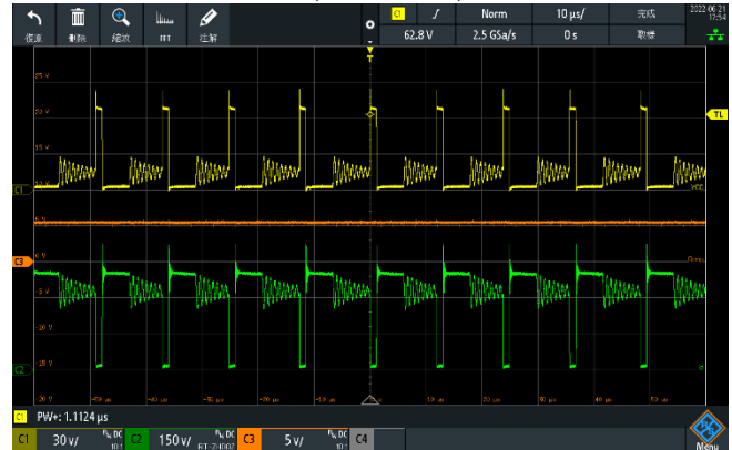
CH1: VDS 30V/div, CH2: Pri_VDS 150V/div, CH3: VDD 5V/div
