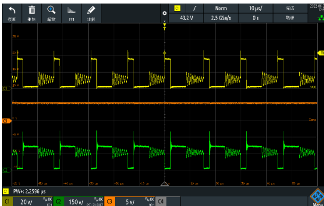
Operating at 65W Flyback Application VIN= 115VAC, VOUT= 9V, IOU= 3A
