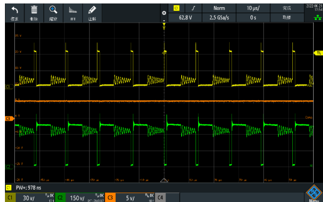
Operating at 65W Flyback Application VIN= 230VAC, VOUT= 9V, IOU= 3A
