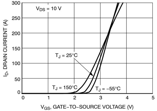
Figure 2. Transfer Characteristics
