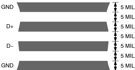
Figure 22. Typical Arrangement of Signal Tracks
