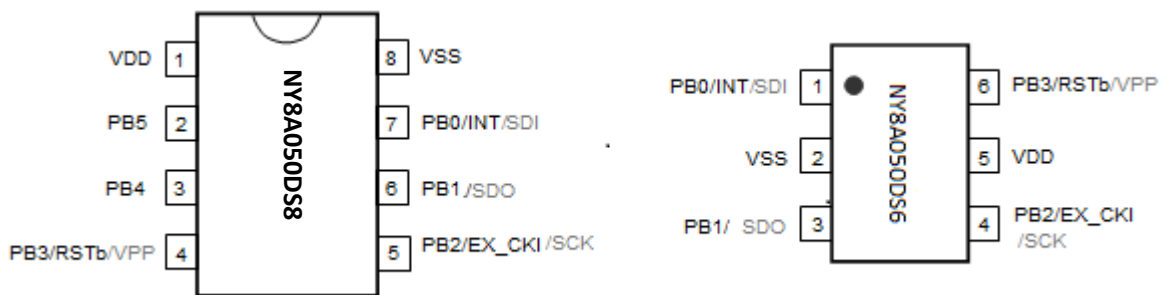
Figure 1 Package pin assignment
