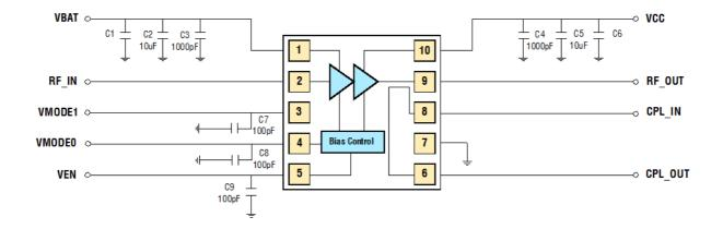
1. RF input and output are 50-Ohm microstrip.
