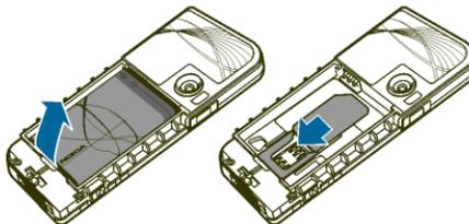
To remove the SIM card press the card release (1) and slide the SIM card towards the top of the phone (2).
