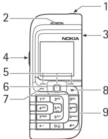
the joystick also functions as the middle selection key, and pressing it briefly selects the function shown on the display above the joystick.
