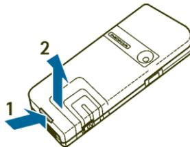
2. Remove the battery by lifting it as shown. Insert the SIM card into the SIM card holder until it snaps into position. Make sure that the SIM card is properly inserted and that the golden contact area on the card is facing downwards.
