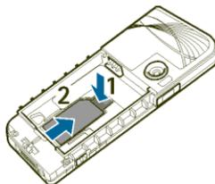
3. Replace the battery. Observe the contacts of the battery
