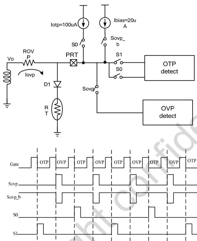
On-Bright proprietary dual function of external OTP and output OVP provides feasible and accurate detection of external OTP through NTC resistor and output OVP. The dual function is realized through time-division technology as shown in the figure.
