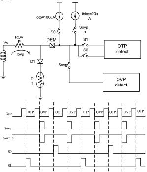
On-Bright proprietary dual function of external OTP and output OVP provides feasible and accurate detection of external OTP through NTC resistor and output OVP. The dual function is realized through time-division technology as shown in the figure.
