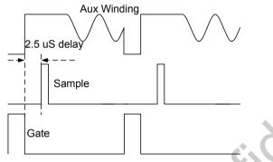
The auxiliary winding voltage is a well-defined replica of the output voltage. The OVP works by sampling the plateau voltage at CS pin during the flyback phase. OB2365D can sample this flat voltage level after a delay time to perform over temperature protection. This delay time is used to ignore the voltage ringing from leakage inductance of PWM transformer.
