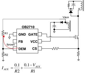
R1: The resistor connected from DEM to AUX. R2: The resistor connected from DEM to ground. When system starts up, if  $I_{AUX} < I_{brown\_in}$ , Brown-in auto-recovery protection is triggered after 2 Gate cycles debounce. When the system enters the
