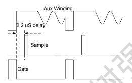
The auxiliary winding voltage is a well-defined replica of the output voltage. The OTP works by sampling the plateau voltage at CS pin during the flyback phase. OB2710 can sample this flat voltage level after a delay time to perform over temperature protection. This delay time is used to ignore the voltage ringing from leakage inductance of PWM transformer.
