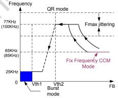
At full load conditions, there are two situations: firstly, if the system input is in low line input range, the IC operates in 85K fixed frequency CCM mode. Thus, small size transformer can be used with high power conversion efficiency. Secondly, if the system input is in high line input range, the IC operates in QR mode. In this way, high power conversion efficiency can be achieved in the universal input range when system is at full loading conditions.
