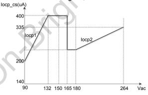
At overload condition when FB input voltage exceeds power limit threshold value for more than Td\_OLP, control circuit reacts to shut down the converter. It restarts when VCC voltage drops below UVLO limit.
