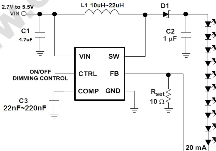
Figure 2, Typical Application Circuit of OCP8178A
