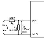
Shunt resistance  $Rs = \frac{Vs}{IIN} \Omega$ It is important to note the power dissipation in the shunt and choose resistor rating accordingly  $Ps = \frac{Vs}{IIN}^2 = IIN^2 Rs \Omega$
