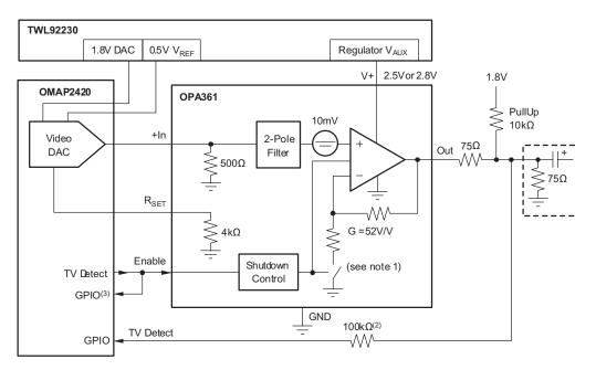
Figure 10. Using TV-Detect Signal to Disable/Enable the OPA361-Q1
