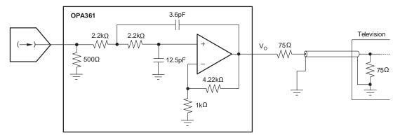
Figure 2. Filter Structure of the OPA361-Q1
