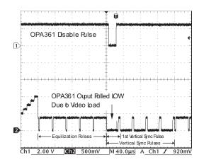
Figure 9. Output of OPA361-Q1 Pulled Down: TV Connected.
