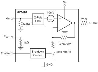
(1) Closed when enabled during normal operation; open when shut down.
