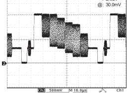
Figure 3. 100/75 Color Bar Signal at Output of OPA361-Q1
