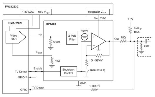
Figure 1. Typical Application using the OMAP242x and the TWL92230
