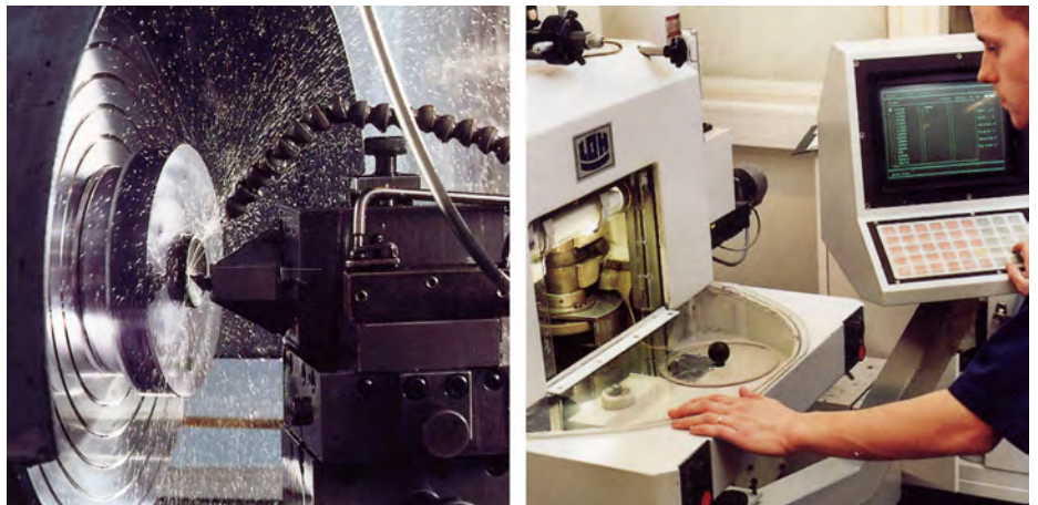
Figure 13.4 LEFT: Diamond turning machine; RIGHT: Lens polishing
