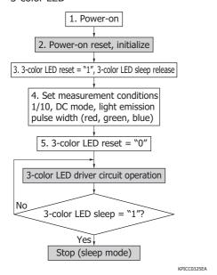
With the initial settings, the 3-color LED driver is in sleep mode. Therefore, first disable the standby mode (3). Next, set the light emission pulse width of each color, 1/10 mode, and the like. Then, release the reset to start measuring (4, 5). 3-color LED drivers continue to operate until they are set to sleep mode. To end operation, enable standby mode.
