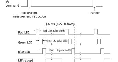
The 3-color LED emits light in the order red, green, and blue. The light emission pulse width can be set in the range of 0  $\mu$ s to 240  $\mu$ s in 16- $\mu$ s steps (16 levels total). The light emission pulse width can be set for each color. The light emission cycle is fixed at approximately 1.6 ms, and the drive current is fixed at 8 mA.
