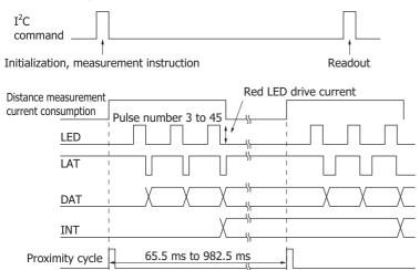
In the proximity sensor, the light emission pulse count is designed to be adjustable in integer multiples of 3 from 3 to 45 in order to increase measurement precision. The interrupt signal (INT) is set to 1 only when all pulses are detected.
