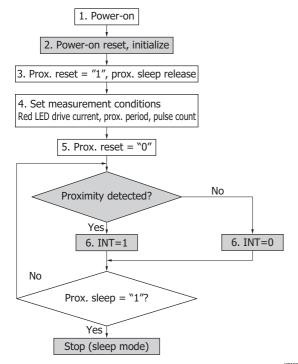
With the initial settings, the proximity sensor is in sleep mode. Therefore, first disable the sleep mode (3.). Next, set the drive current, pulse count, pulse cycle, and the like. Then, release the reset to start measuring (4. 5.). Proximity sensor continues to measure until it is set to sleep mode. To end measurement, enable sleep mode.
