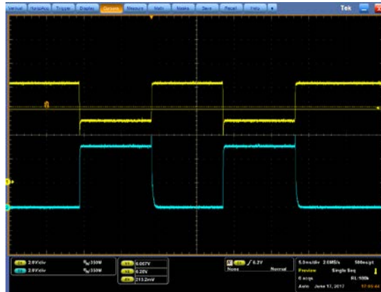
Fig3. OVP recovery waveform (OVP 6V)
