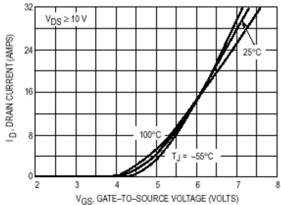
Figure 2. Transfer Characteristics
