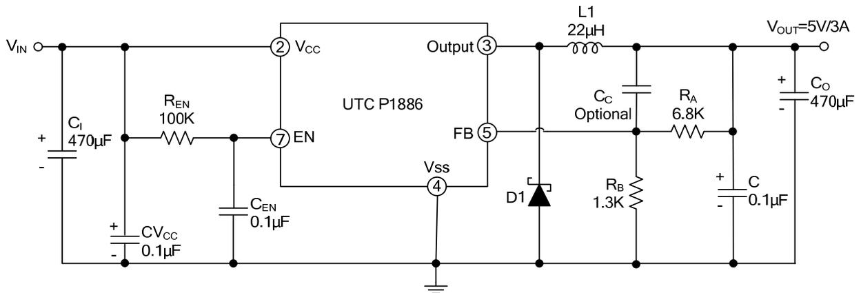
Note:  $V_{OUT} = V_{FB} \times (1 + R_A/R_B)$ ,  $R_B = 0.7K \sim 5K \text{ ohm}$
