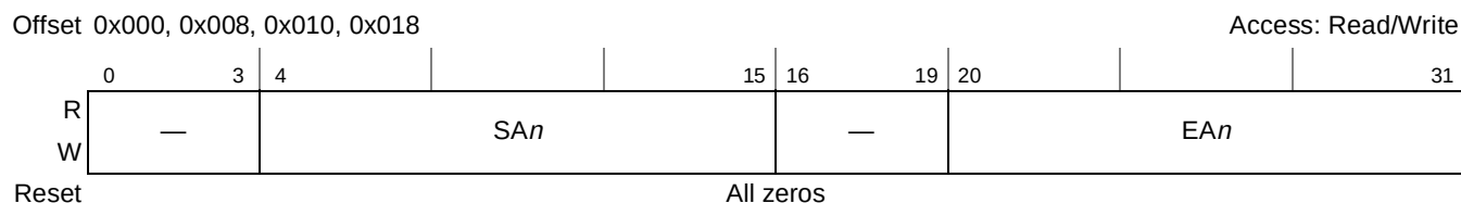
Figure 8-2. Chip Select Bounds Registers ( CS_n\_BNDS )
