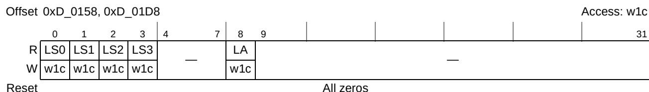
Figure 15-49. Port n Serial Link Command and Status Register (PnSLCSR)
