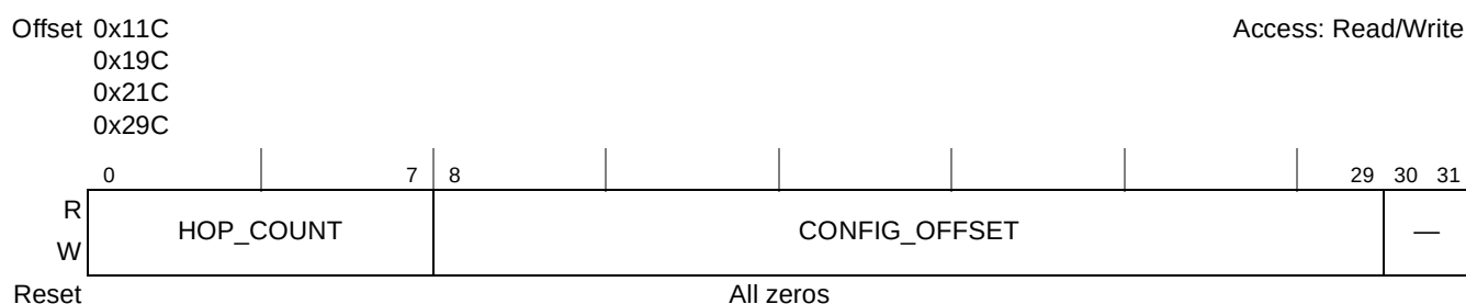
Figure 13-14. Destination Address Registers for RapidIO Maintenance Writes (DARN)
