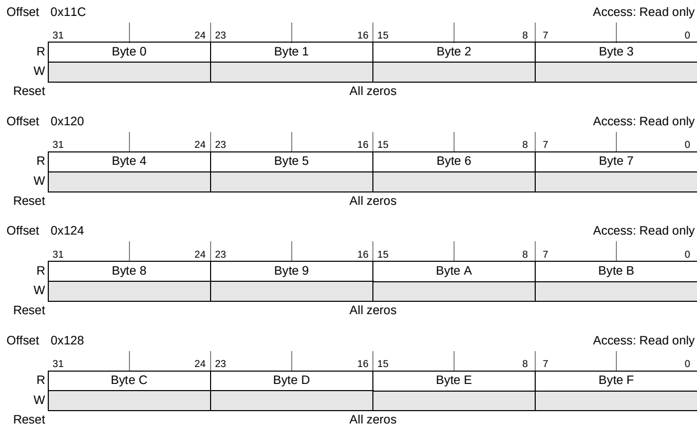
Figure 16-110. PCI Express Header Log Register
