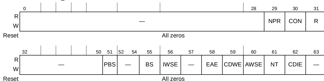
Figure 20-11. Channel Configuration Register (CCR)
