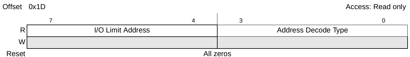
Figure 16-65. PCI Express I/O Limit Register
